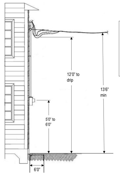
(2) 5/8" x 8'0" copper clad ground rod to be flush with or below grade in undisturbed soil
